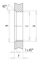
Installation direction: o-ring sits on chamfer.
